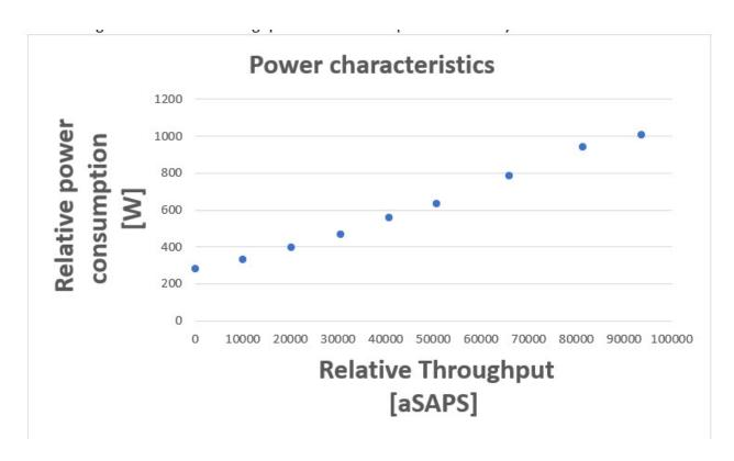
Linear power consumption is important for servers to enable accurate workload scheduling, optimize data center cooling and power infrastructure, and facilitate energy management and cost savings. While real-world server power consumption isn't always perfectly linear, a linear model provides a simple, accurate approximation essential for predicting energy usage, identifying inefficiencies, and making informed decisions about server and data center operations.
