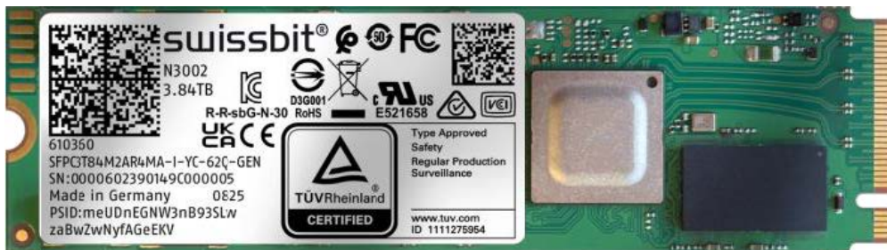
Figure 1. ThinkSystem M.2 N3002 Read Intensive NVMe PCIe 4.0 Industrial SSDs
