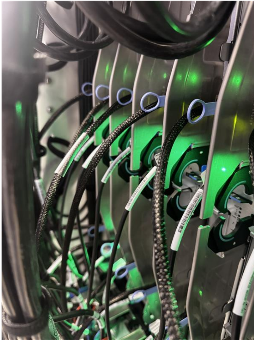
Figure 8: Side view of a full 16 node N1380 DWC enclosure connected over a CN5000 Omni-Path network (cables with the blue tab).
