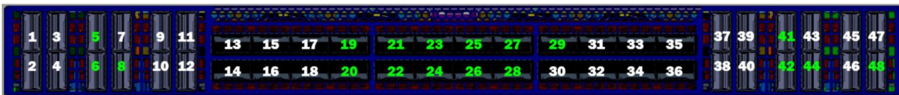
Figure 10: CN5000 Switch with “Extended reach ports” highlighted in green. Taken from Cornelis Network CN5000 cabling guidance document [2].
