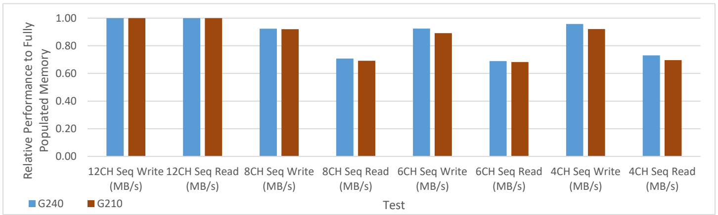
Figure 15 Sequential Read and Write Throughput measured on DSS-G210 and G240 with memory channels on the controllers depopulated.
