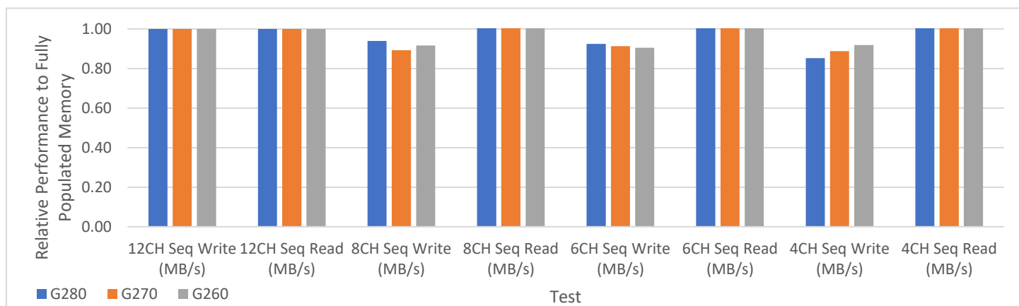
Figure 14 Sequential Read and Write Throughput measured on DSS-G270 and G280 with memory channels on the controllers depopulated.
