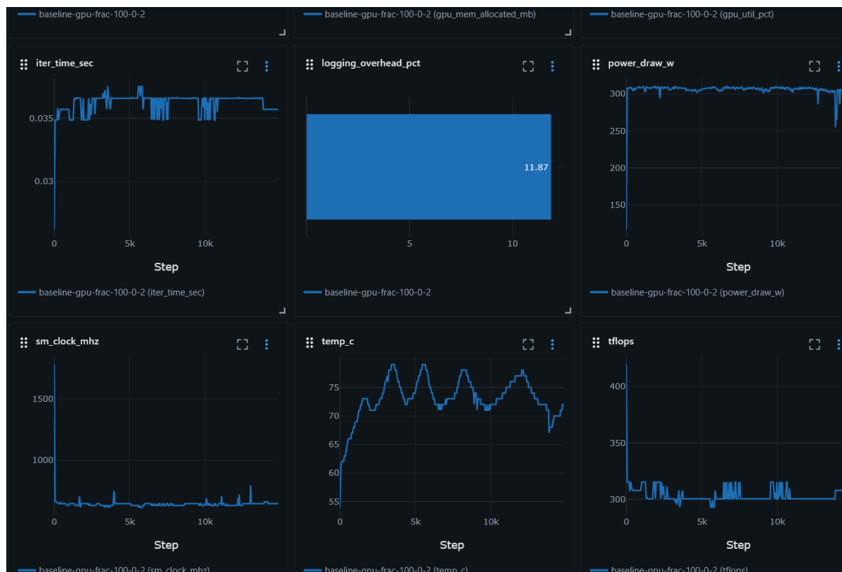
Figure 14. Live GPU telemetry captured in MLflow during a sustained workload, including power draw, clock speed, temperature, and achieved throughput.
