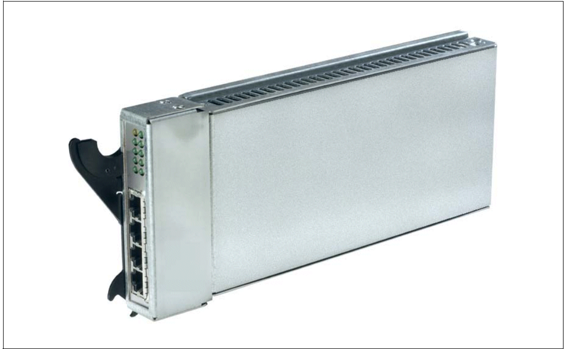
Figure 1-10 BladeCenter 4-Port Ethernet Switch Module
