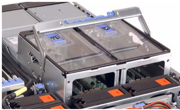
The memory cassette partially removed from the server chassis (eight-DIMM board). The clear plastic doors open for easy access to DIMMs.
