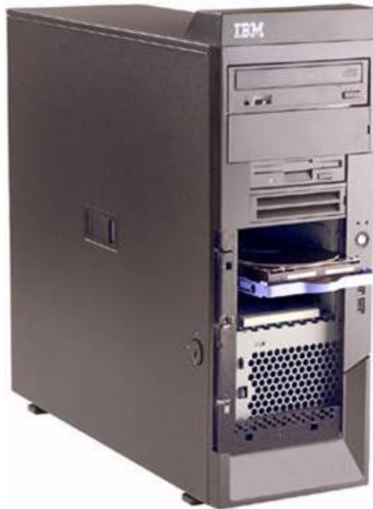
Figure 3-7 Front accessible simple-swap SATA drives (x206)
