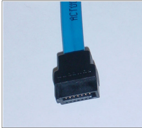
Figure 3-5 SATA cable and connector
