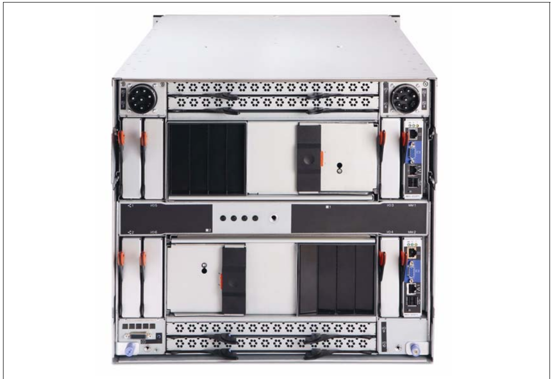
Figure 1-3 BladeCenter H rear view
