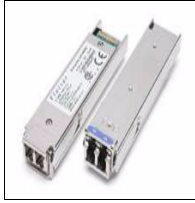
Figure 4-2 XFP (10 Gigabit Small Form Factor Pluggable) options
