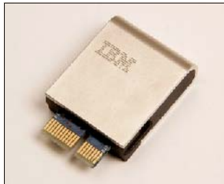
Figure 1-5 ScaleXpander Option Kit component to enable multinode configurations
