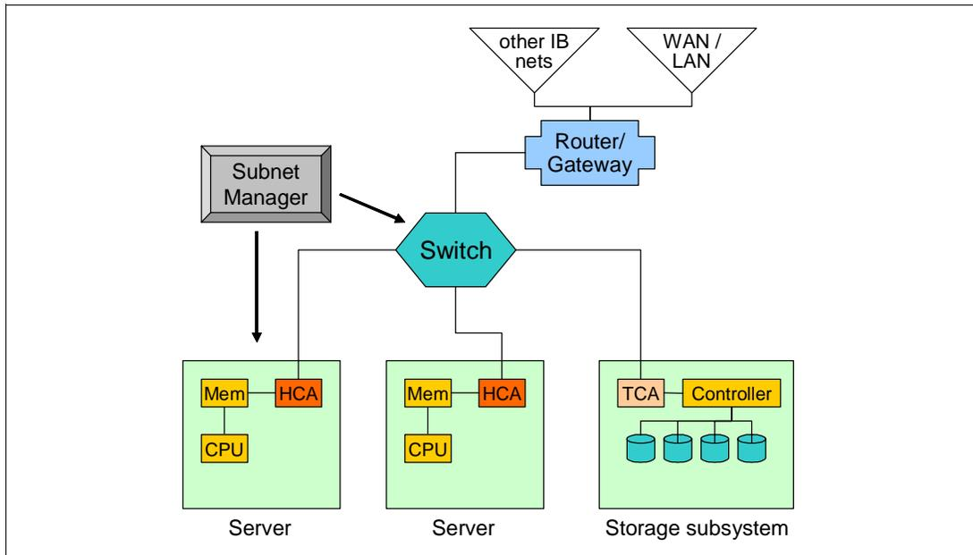
Figure 1 Elements of an InfiniBand network
