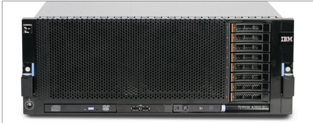
Figure 3-24 Front view of the x3850 X5 showing eight 2.5-inch SAS drives
