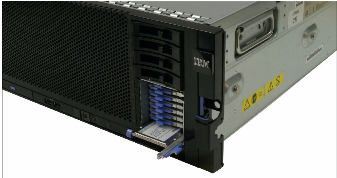
Figure 3-25 IBM eXFlash with eight SSDs
