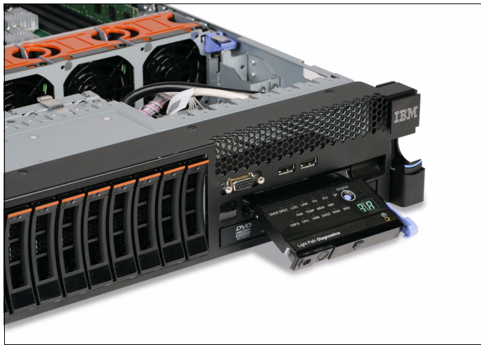
Figure 4-46 x3690 X5 light path diagnostics panel
