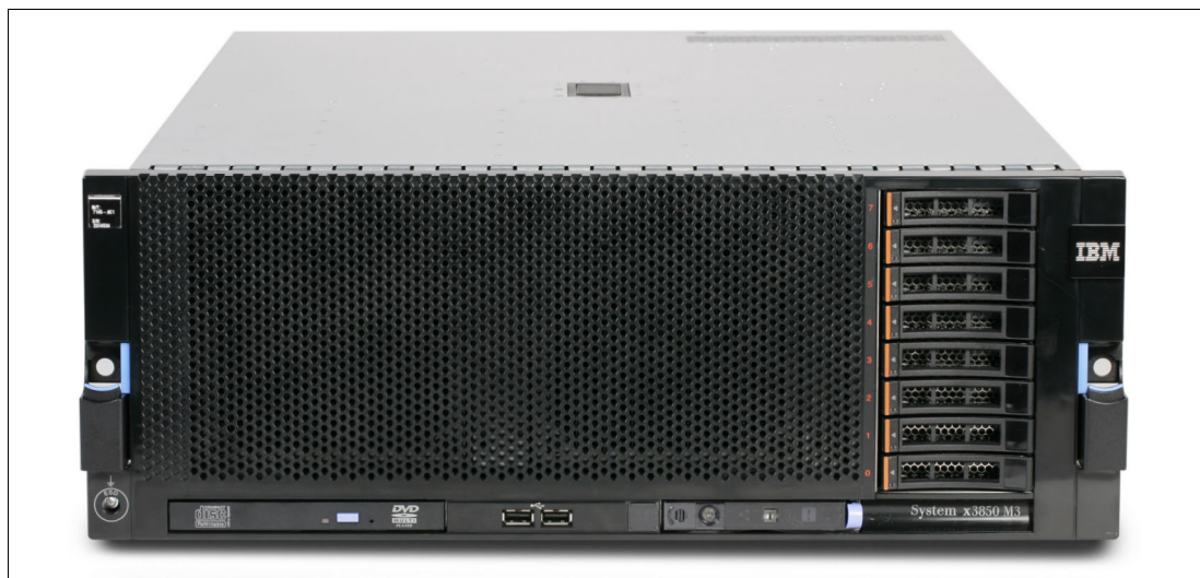
Figure 3-1 Front view of the x3850 X5 showing eight 2.5-inch SAS drives
