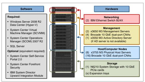
Figure 2 Major components of the System x Private Cloud Offering (Advanced configuration)
