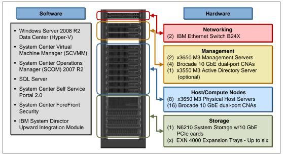
Figure 1 Major components of the System x Private Cloud Offering (Mainstream configuration)
