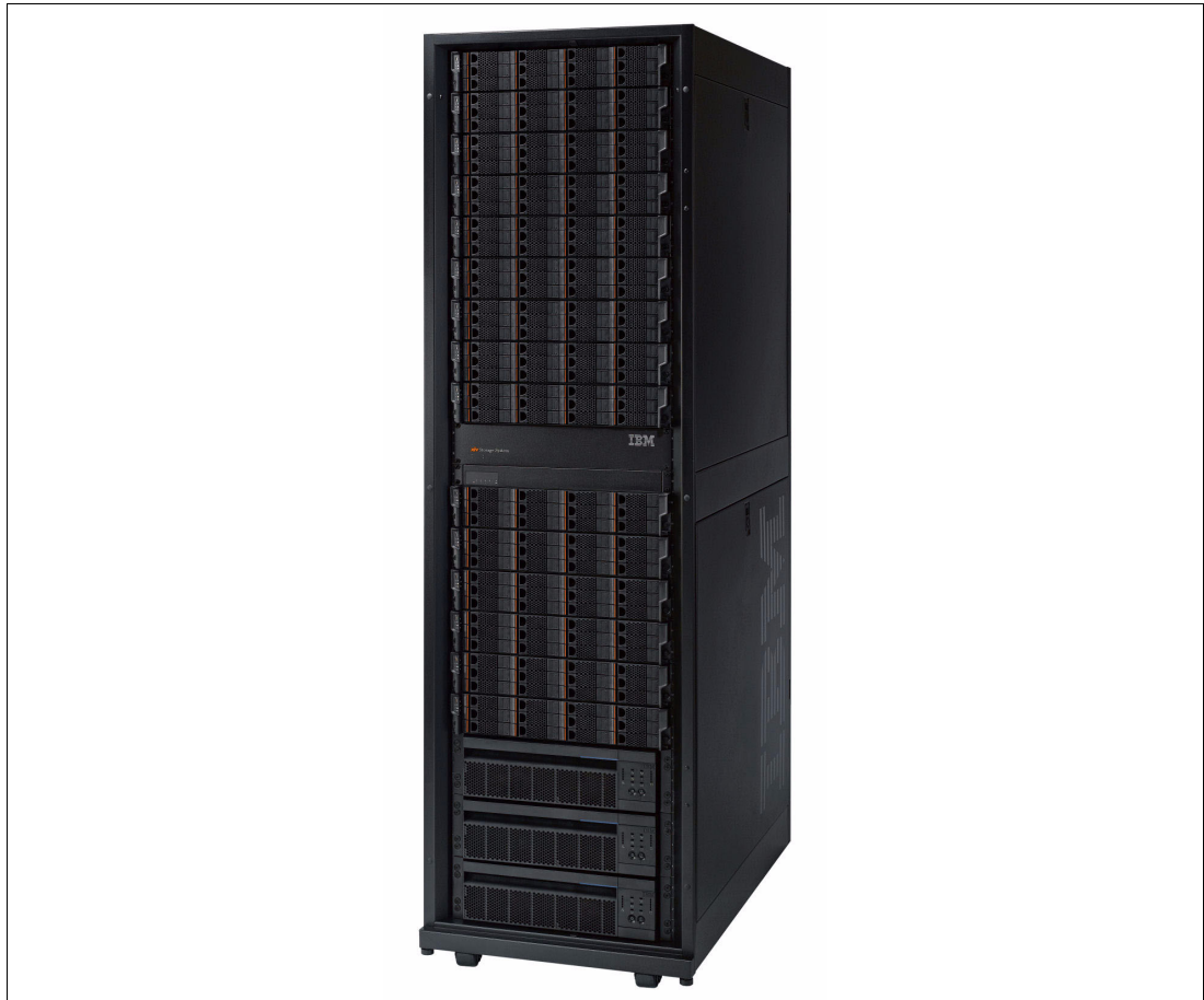
Figure 2 IBM XIV Storage System
