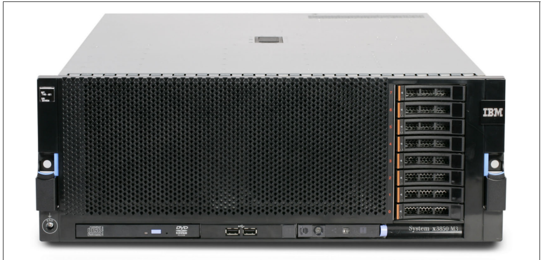
Figure 1 Front view of the x3850 X5 showing eight 2.5-inch SAS drives
