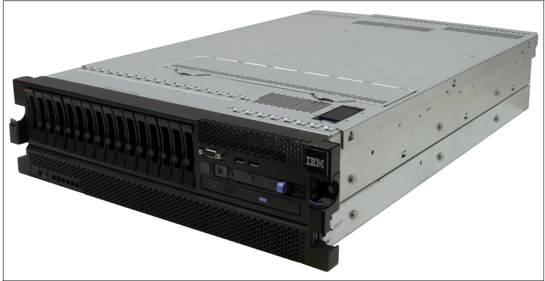
Figure 1 IBM System x3690 X5 with MAX5 memory expansion unit attached beneath it
