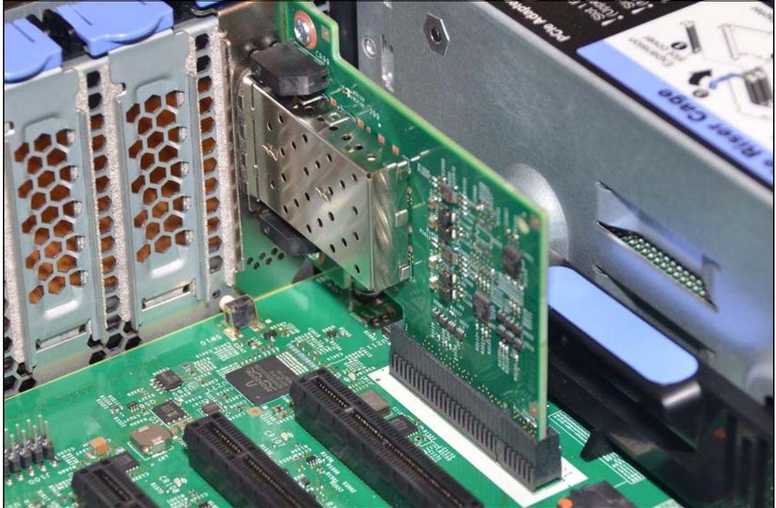
Figure 1-41 10 GbE adapter in the dedicated connector (machine type 8722)
