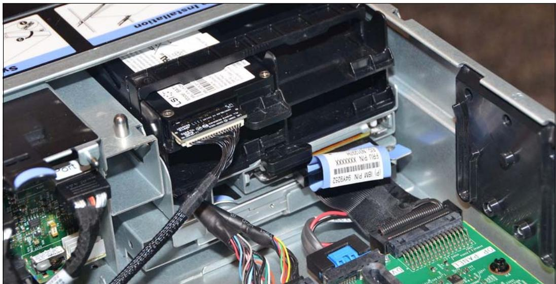
Figure 1-38 *Battery and flash power module tray (system fans removed)*
