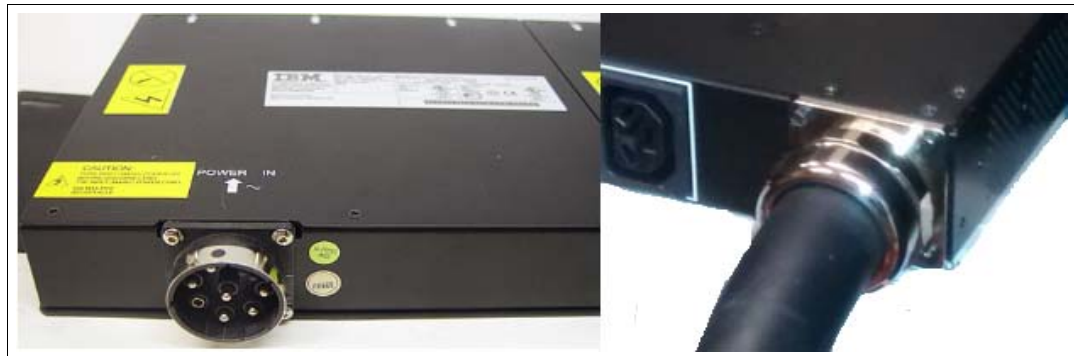
Figure 2-15 AC PDU with a detachable line cord and an HVDC PDU with a hardwired line cord
