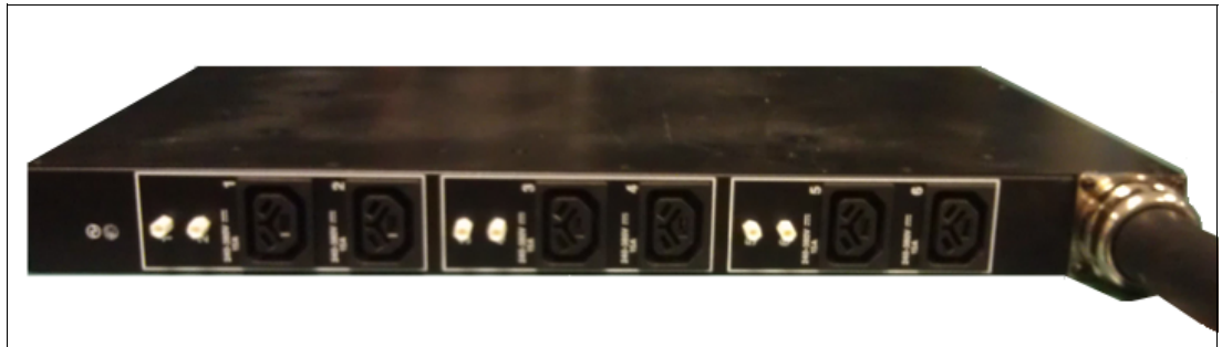
Figure 4-9 HVDC PDU front
