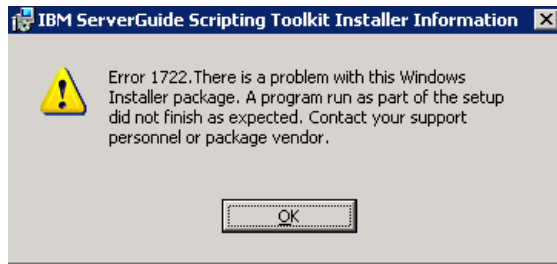
Figure 2-17 Error message when installing the SGTK to a drive other than C:
