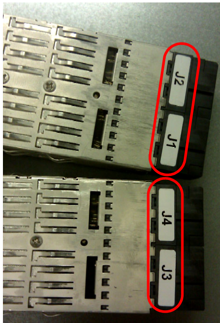
Figure 6-14 QPI cable end labels: J1 and J2 attach to the primary node
