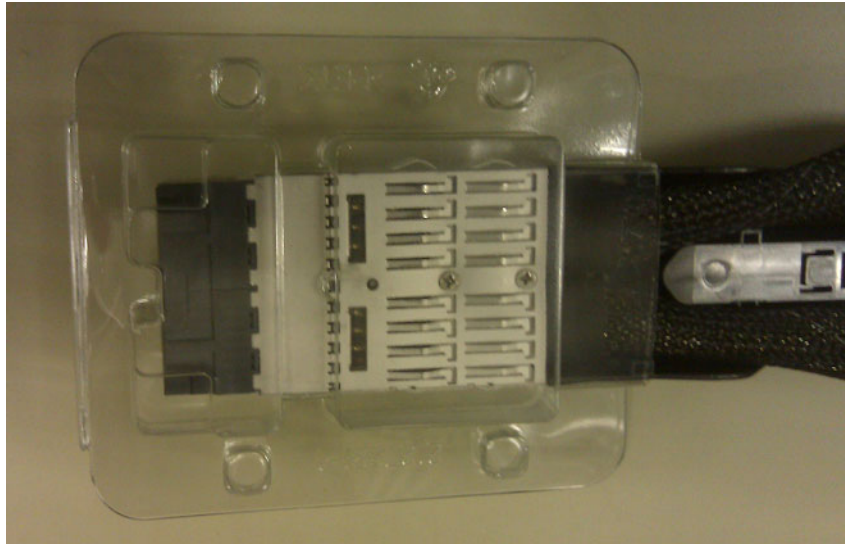
Figure 6-7 Reusable QPI cable connector protective boot
