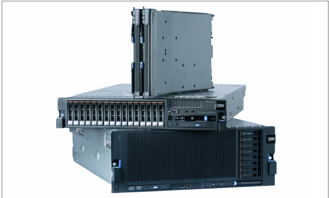
Figure 1-1 eX5 family (top to bottom): BladeCenter HX5 (2-node), System x3690 X5, and System x3850 X5 (the System x3950 X5 looks the same as the x3850 X5)
