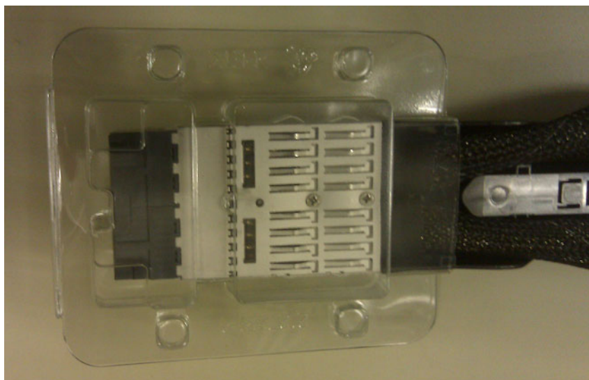
Figure 7-9 Reusable QPI cable connector protective boot
