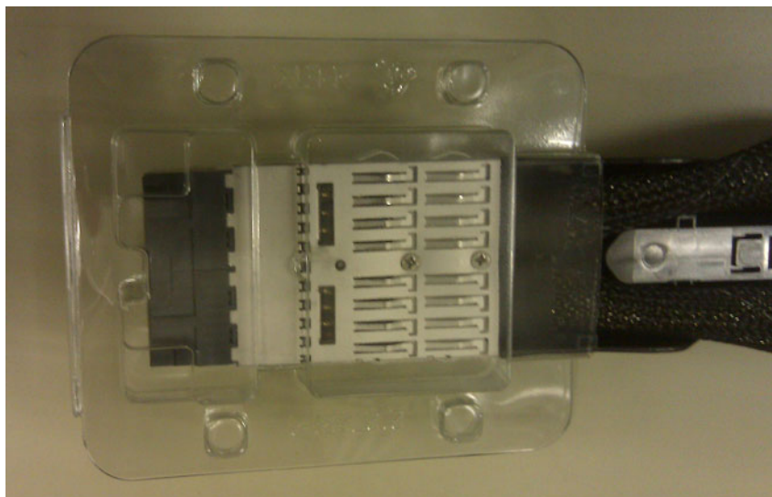
Figure 6-12 Reusable QPI cable connector protective boot
