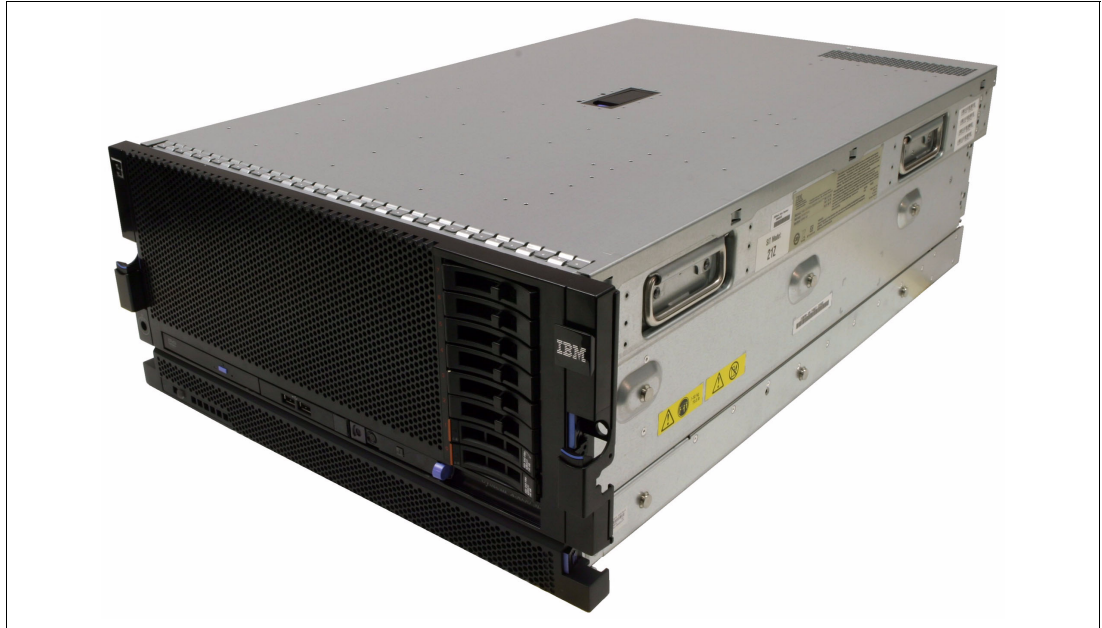
Figure 2-10 IBM System x3850 X5 with MAX5 (the MAX5 is the 1U unit beneath the main system)
