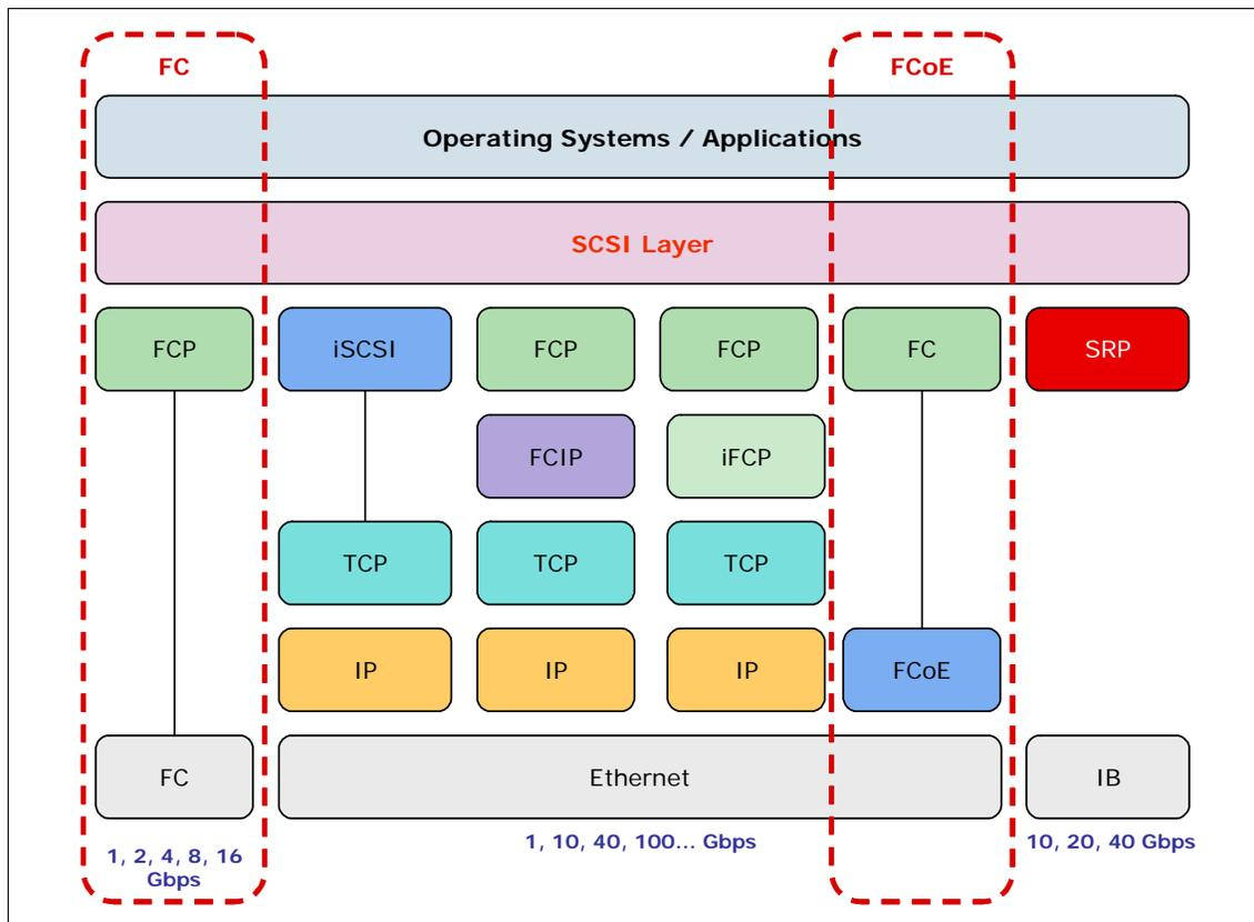
Figure 2-2 Storage Network Protocol Layering
