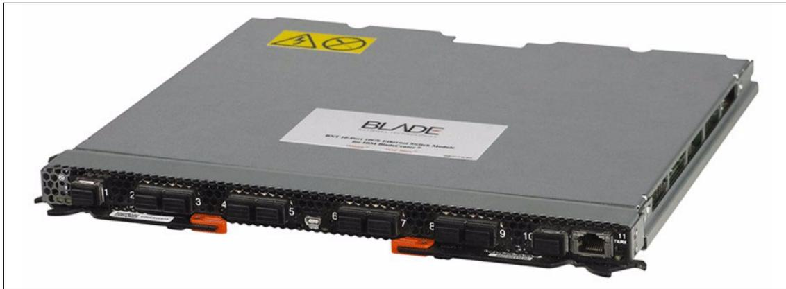
Figure 4-4 BNT Virtual Fabric 10Gb Switch Module
