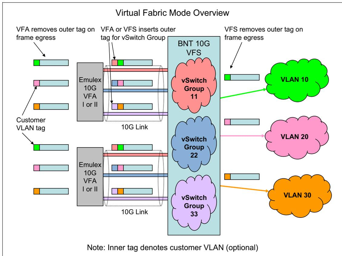
Figure 3-1 Overview of IBM Virtual Fabric Mode
