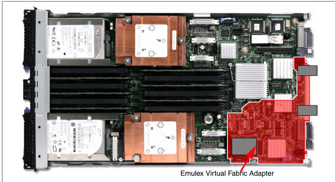
Figure 4-2 Emulex Virtual Fabric Adapter placement in HS22 blade server
