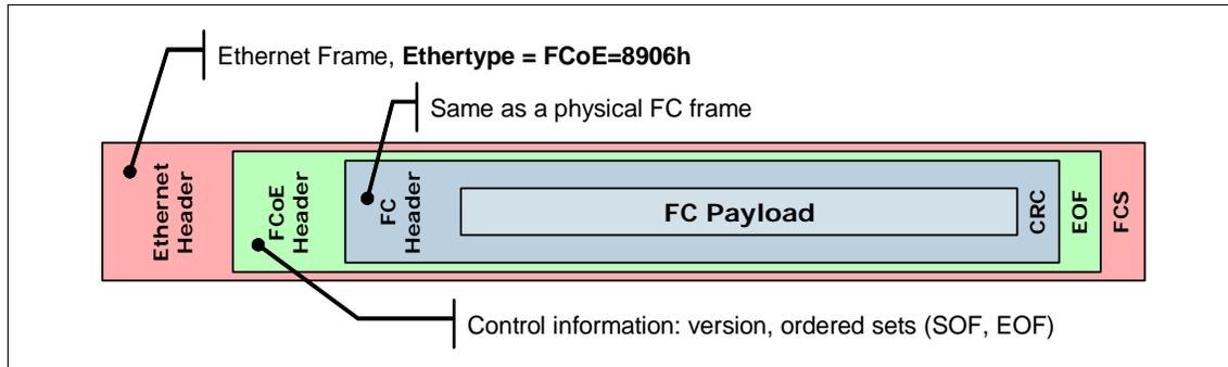
Figure 2-3 Conceptual view of an FCoE frame
