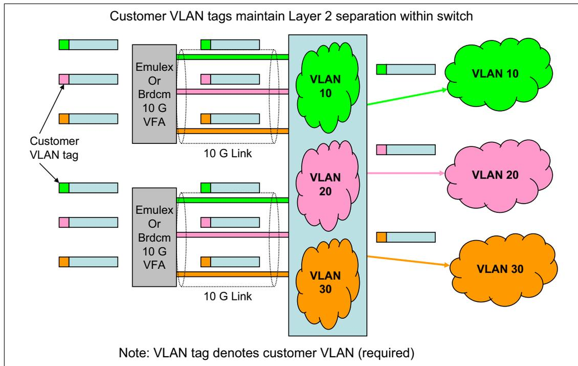
Figure 7-1 Overview of Switch Independent Mode
