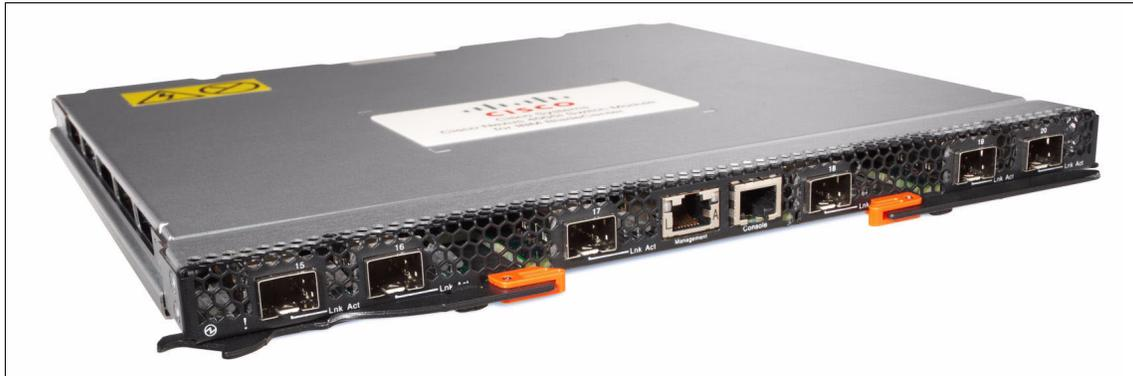
Figure 8-5 Cisco Nexus 4001I Switch Module
