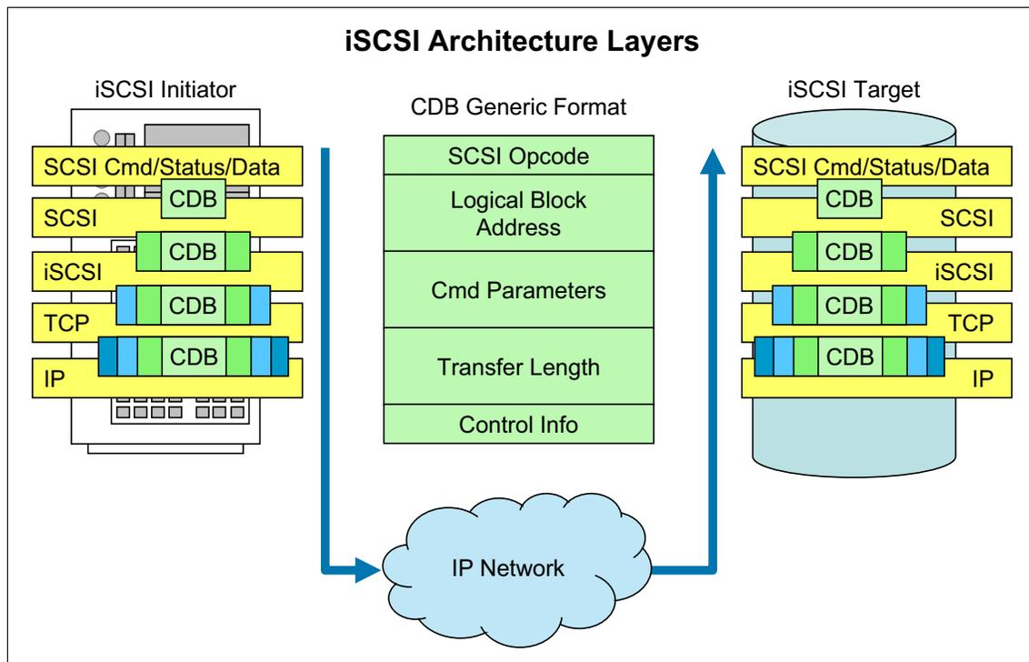
Figure 3-4 iSCSI protocol layers
