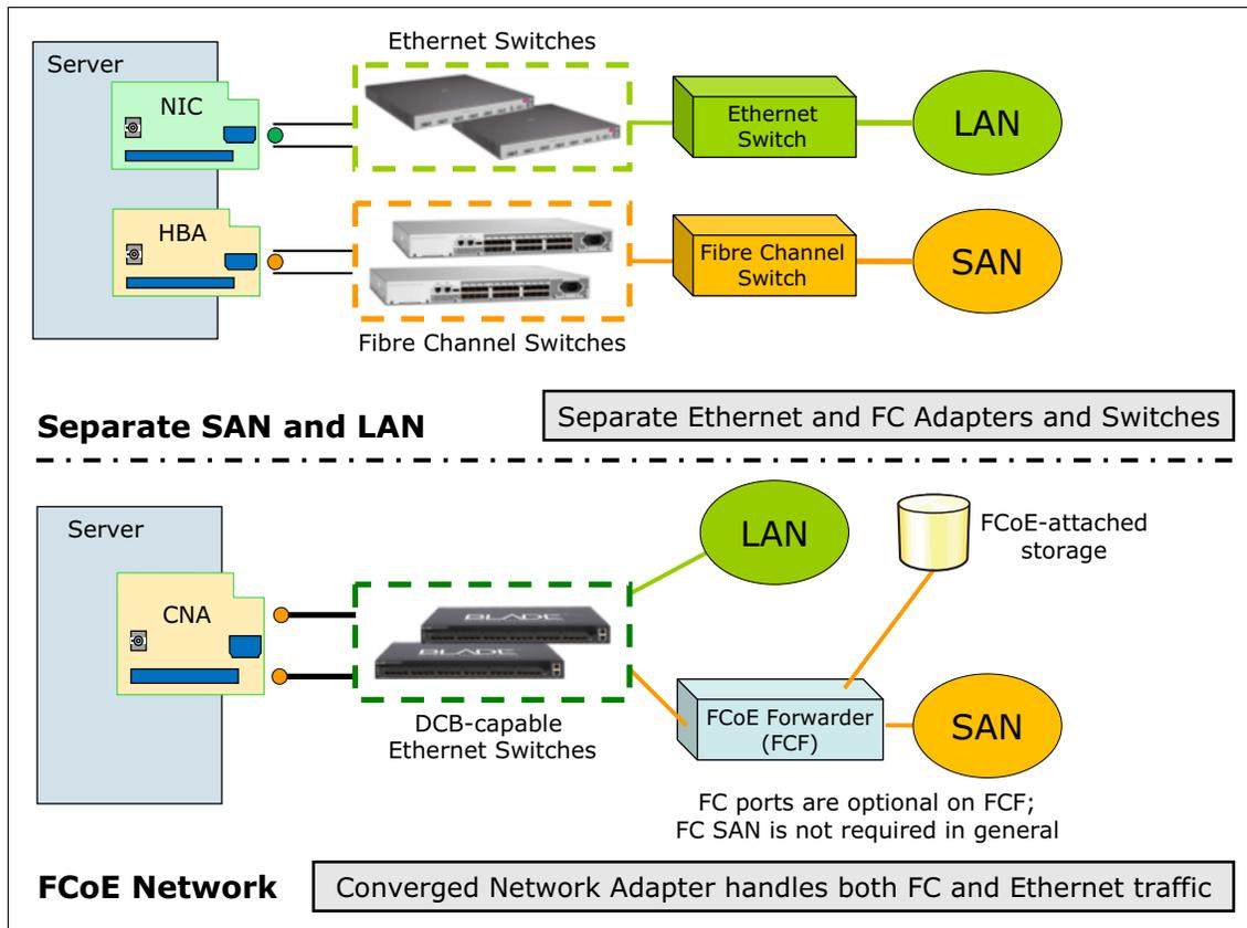
Figure 3-3 Converged Network Adapter (CNA) in a server
