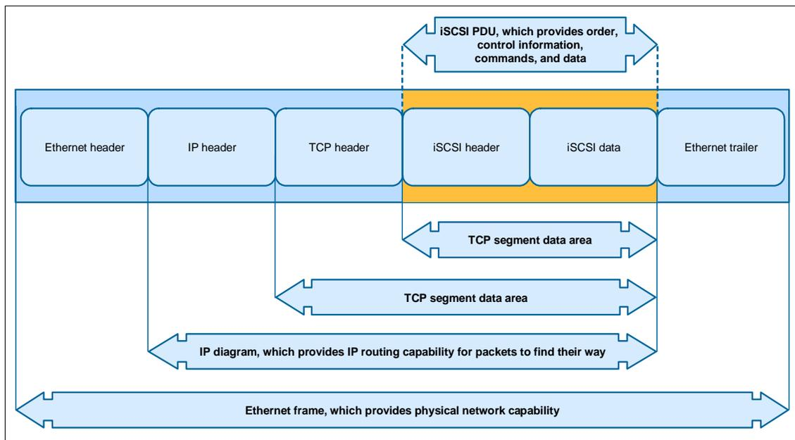
Figure 3-5 iSCSI encapsulation overview
