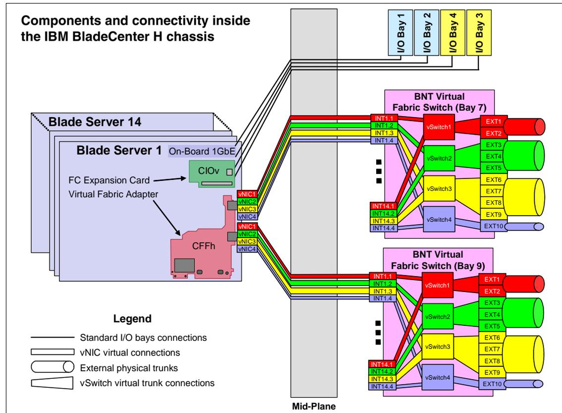
Figure 3-2 BladeCenter Virtual Fabric vNIC solution
