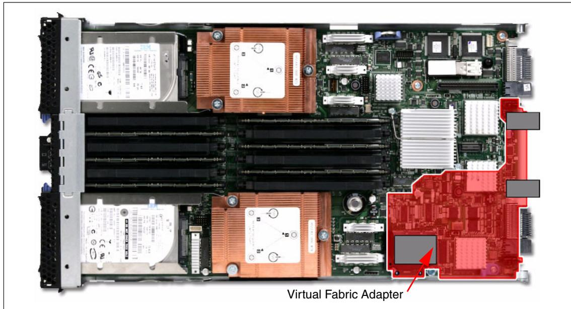
Figure 8-2 Placement of a CFFh card in the BladeCenter HS22 server
