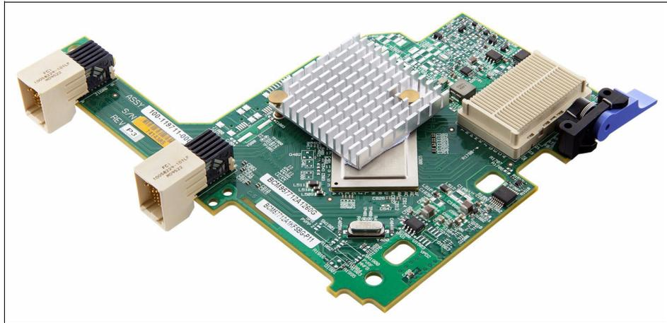
Figure 8-3 Broadcom 2-port 10Gb Virtual Fabric Adapter
