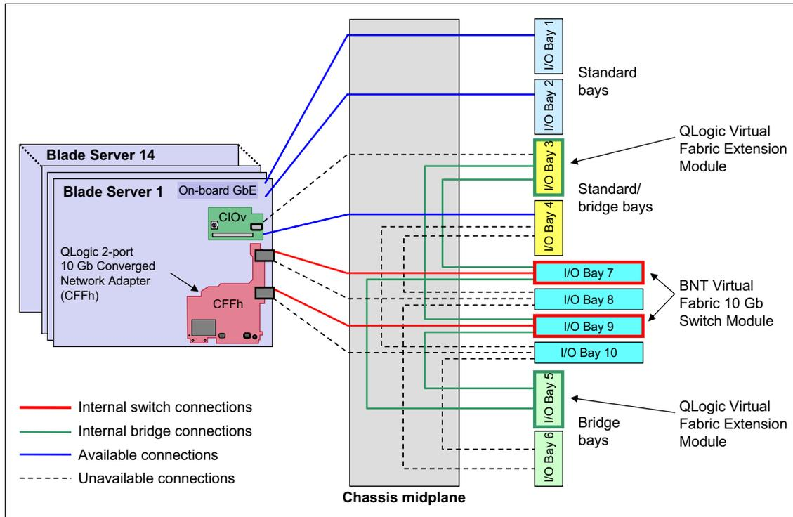
Figure 6-21 BladeCenter H internal connections with the QLogic Virtual Fabric Extension Modules
