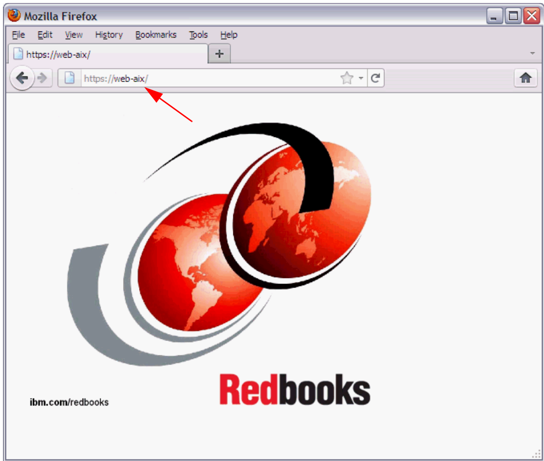
Figure 5-8 Home page on Web server using a secure connection (HTTPS on port 443)
