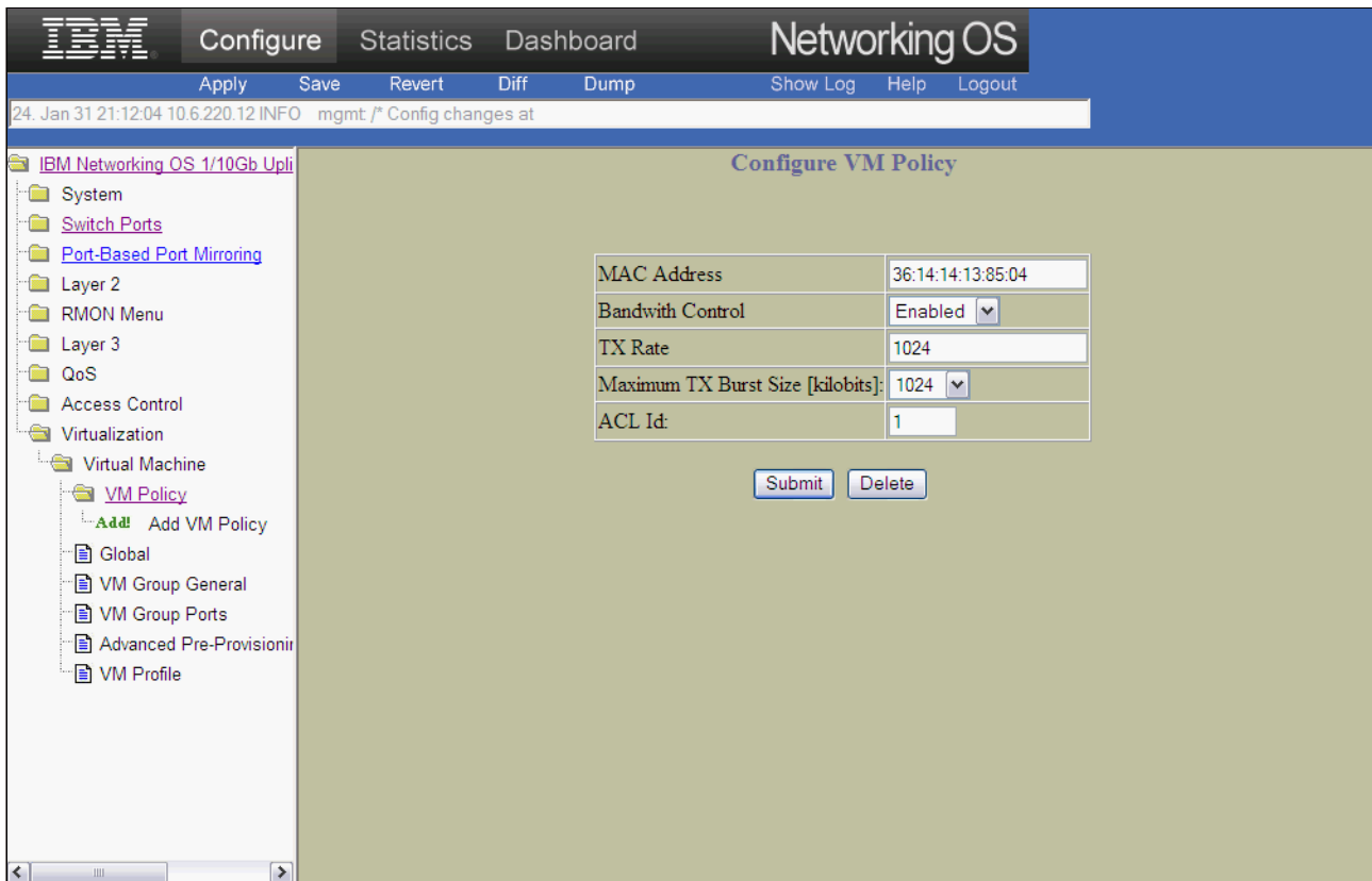
Figure 5-23 Traffic shaping configuration
