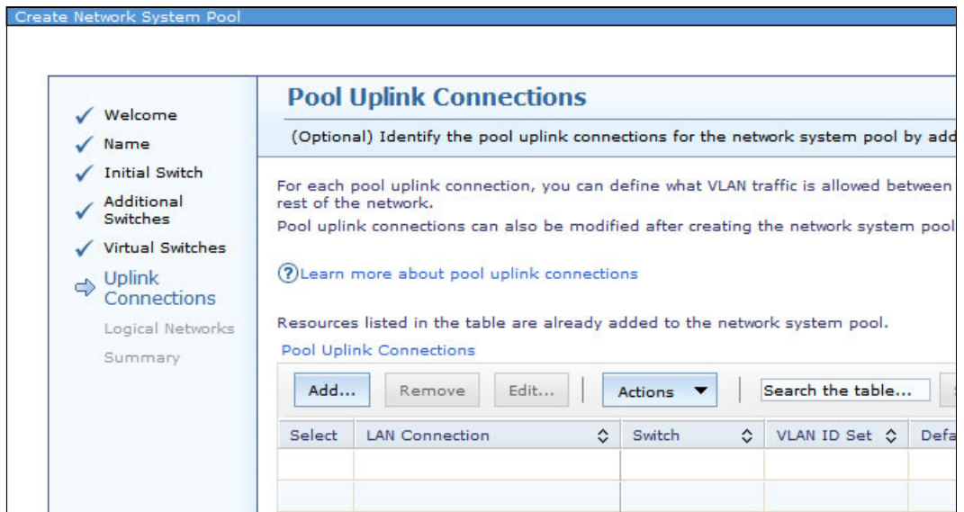
Figure 9-84 Create Network System Pool: Pool Uplink Connections
