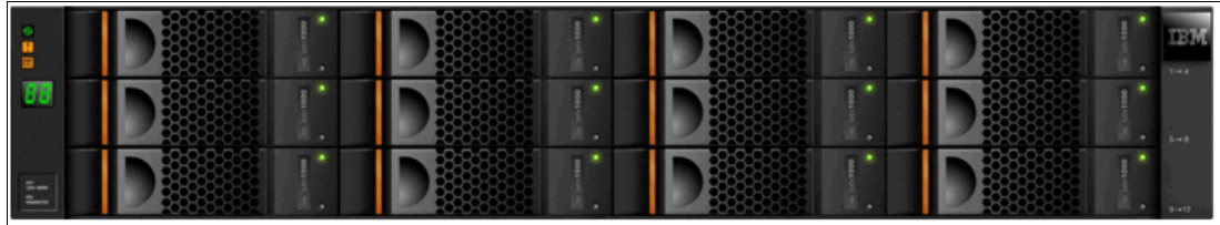
Figure 2-10 IBM Storwize V7000 front view for 2076-212 enclosure
