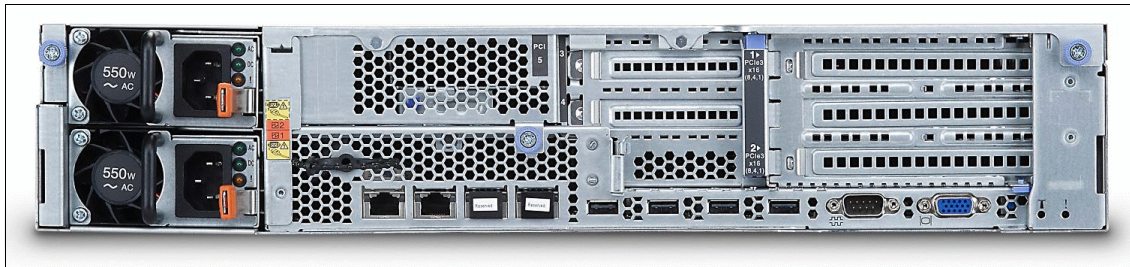
Figure 4-6 Rear view of x3630 M4 without the storage-rich option. See the extra LP PCIe slot (left) and FHHL PCIe slot (right)
