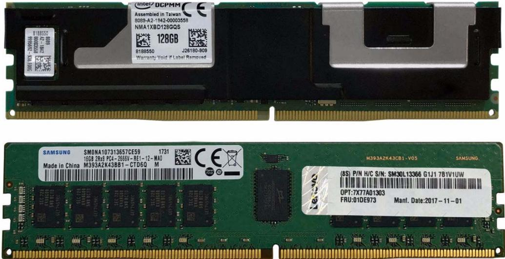
Figure 5-11 Intel Optane DC Persistent Memory Module (top) and Lenovo TruDDR4 DIMM (bottom)
