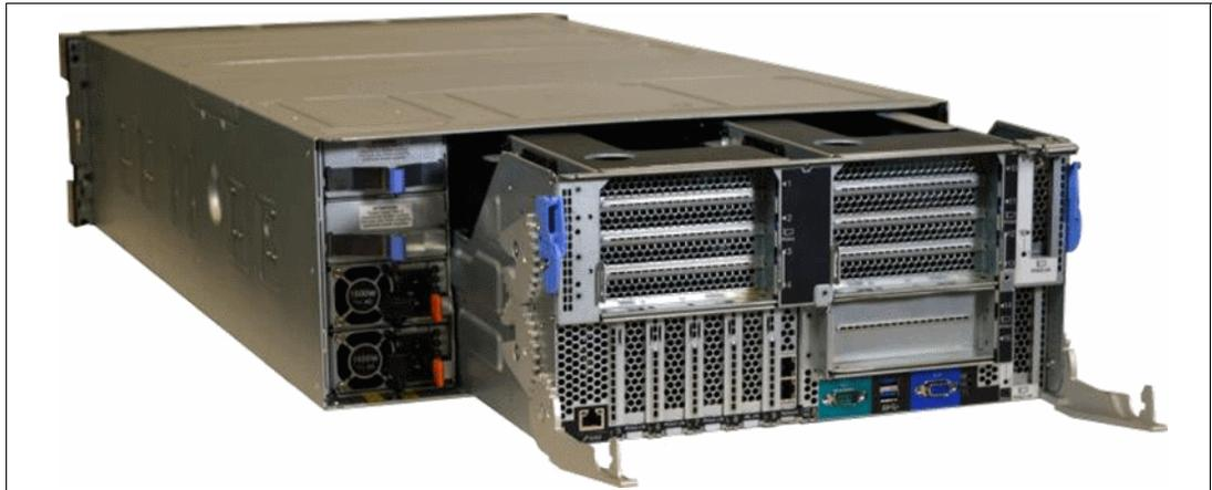
Figure 5-9 I/O tray being removed from the rear of the server
