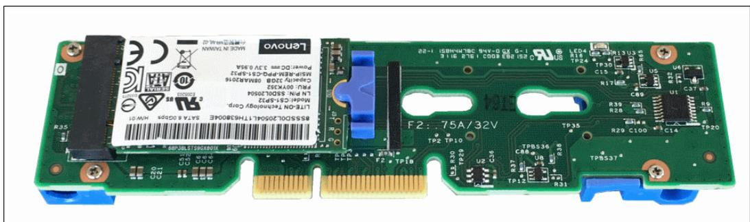
Figure 5-15 Single M.2 Boot Adapter and a 32 GB M.2 drive
