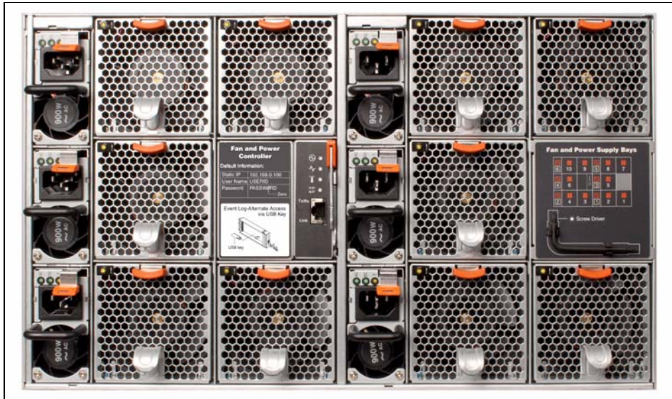
Figure 1-2 Rear of NeXtScale n1200 Enclosure with 900 W power supplies shown
