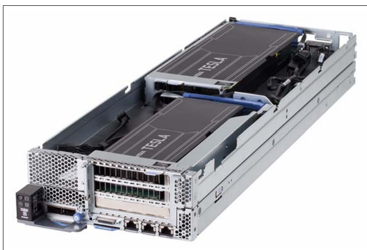
Figure 4-29 NeXtScale PCIe Native Expansion Tray attached to an nx360 M4 compute node
