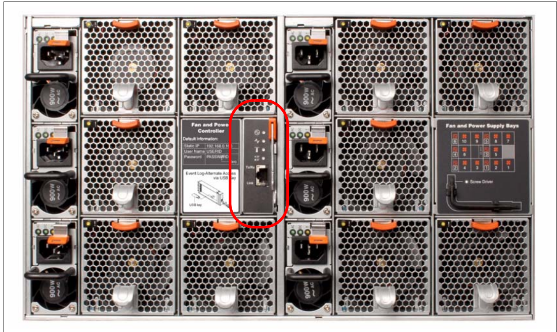
Figure 3-12 Rear view of the chassis that shows the location of the FPC
