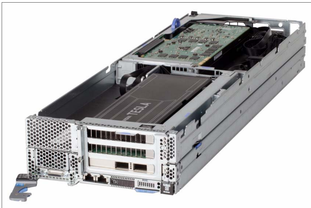
Figure 4-11 NeXtScale PCIe Native Expansion Tray attached to an nx360 M5 compute node
