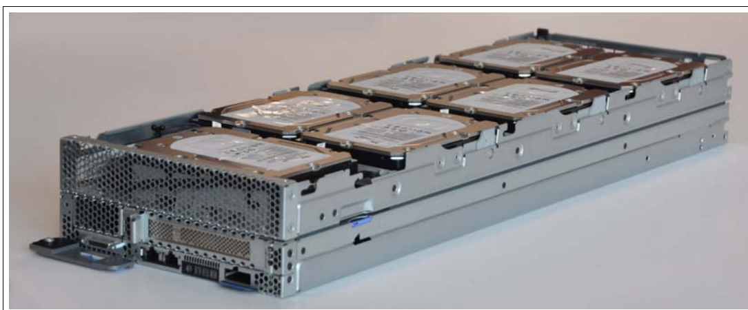
Figure 4-6 NeXtScale 12G Storage Native Expansion Tray attached to an nx360 M5 compute node
