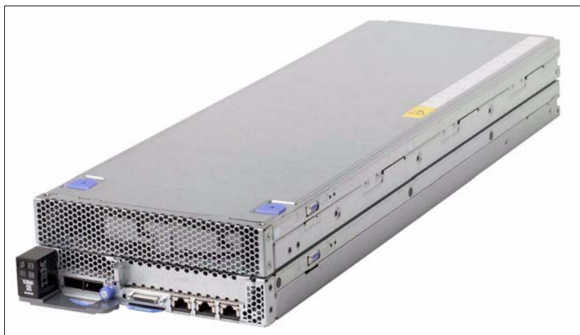
Figure 4-26 NeXtScale Storage Native Expansion Tray attached to an nx360 M4 compute node
