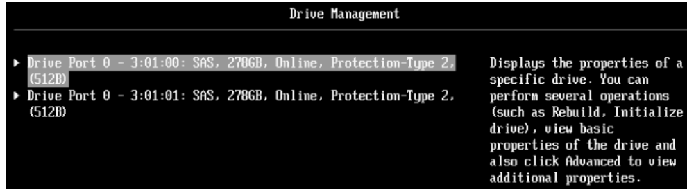
Figure 5-26 Drive Management panel
