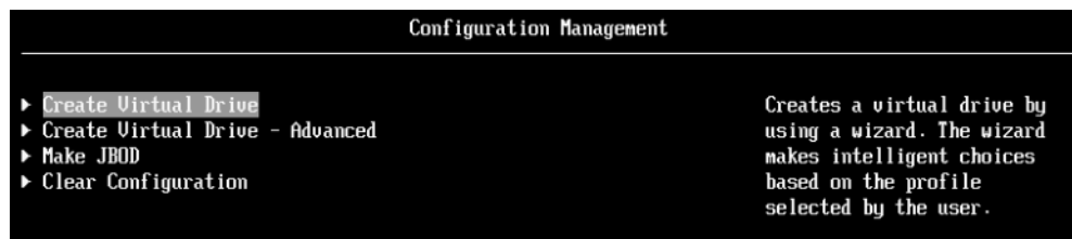
Figure 5-28 Configuration Management panel
