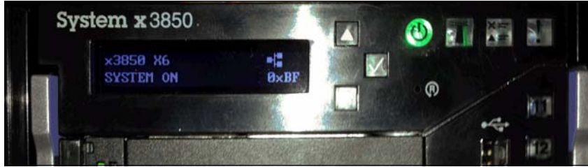
Figure 5-7 LED light path diagnostic panel
