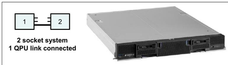
Figure 3-5 QPI connections in a 2-socket configuration
