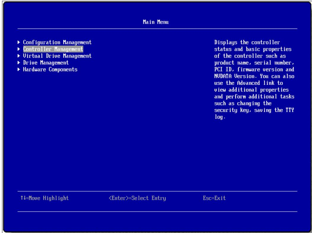
Figure 5-19 LSI MegaRAID Configuration Utility, Main Menu panel
