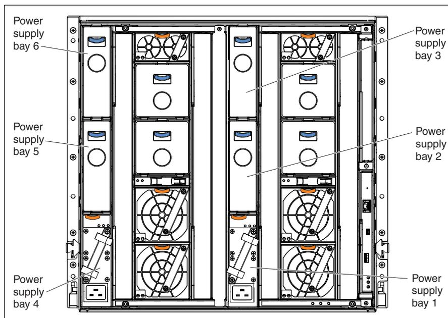
Figure 2-5 Enterprise Chassis power supply locations
