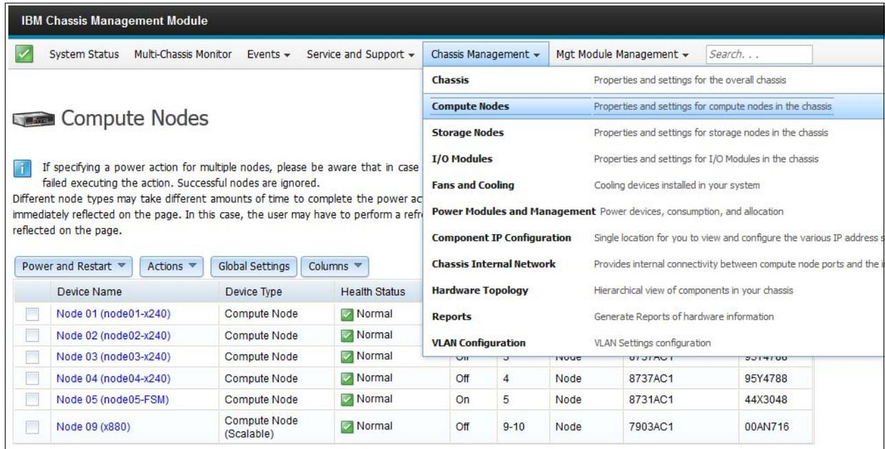
Figure 7-18 Chassis Management Compute Nodes menu
