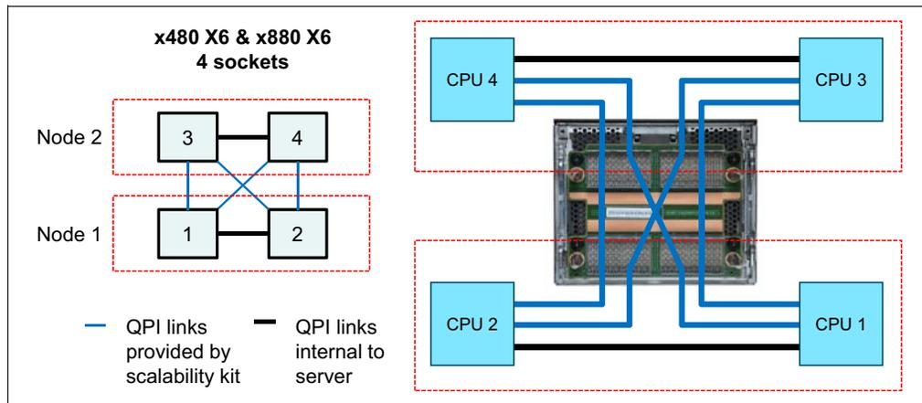
Figure 3-7 QPI connections in a 4-socket configuration
