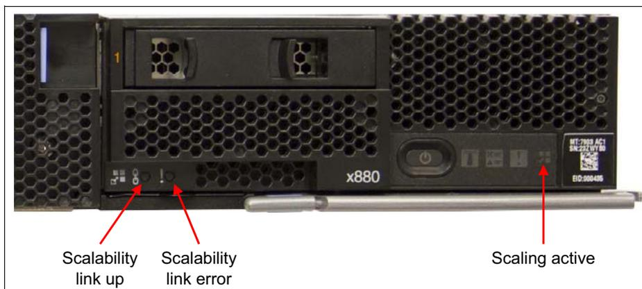
Figure 4-8 Scalability LEDs
