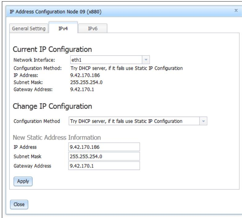
Figure 7-16 Configuring IPv4 information for an IMM
