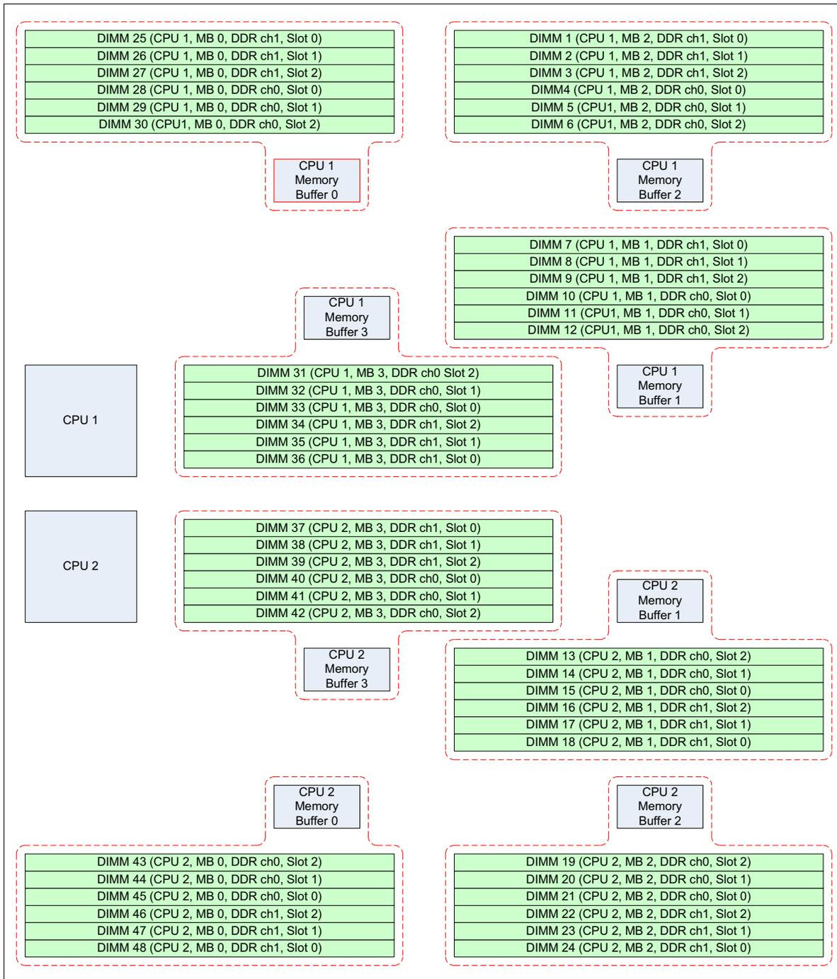
Figure 4-9 DIMM numbering on the x6 system board
