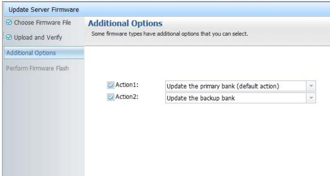
Figure 6-24 IMM Firmware Action panel
