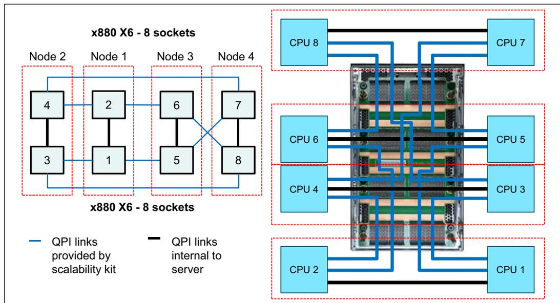
Figure 3-9 QPI connections in an 8-socket configuration
