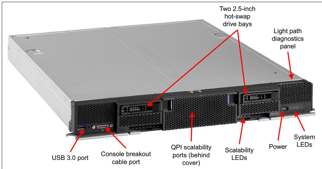
Figure 4-2 The Lenovo Flex System X6 Compute Node
