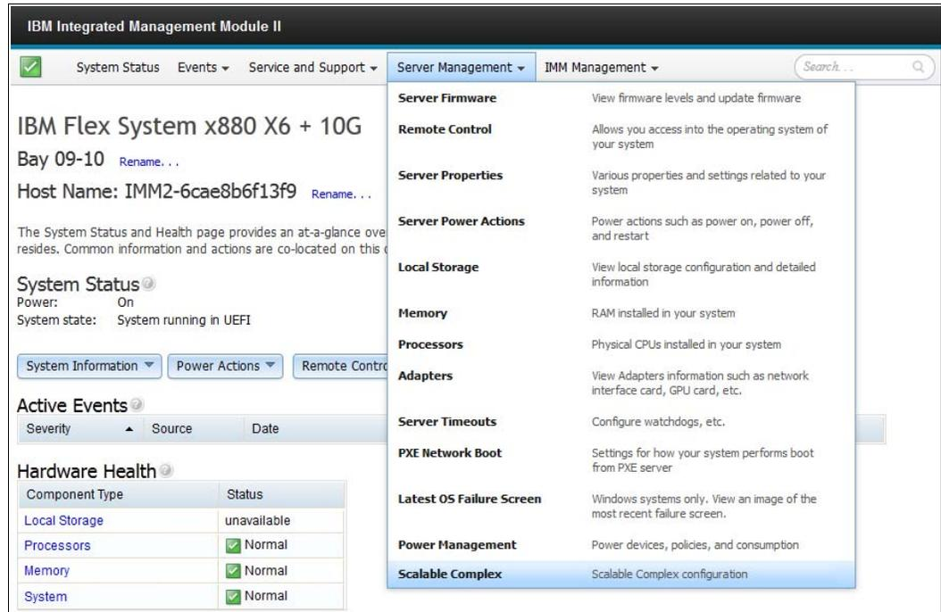
Figure 5-37 Scalable complex server management in IMM web interface
