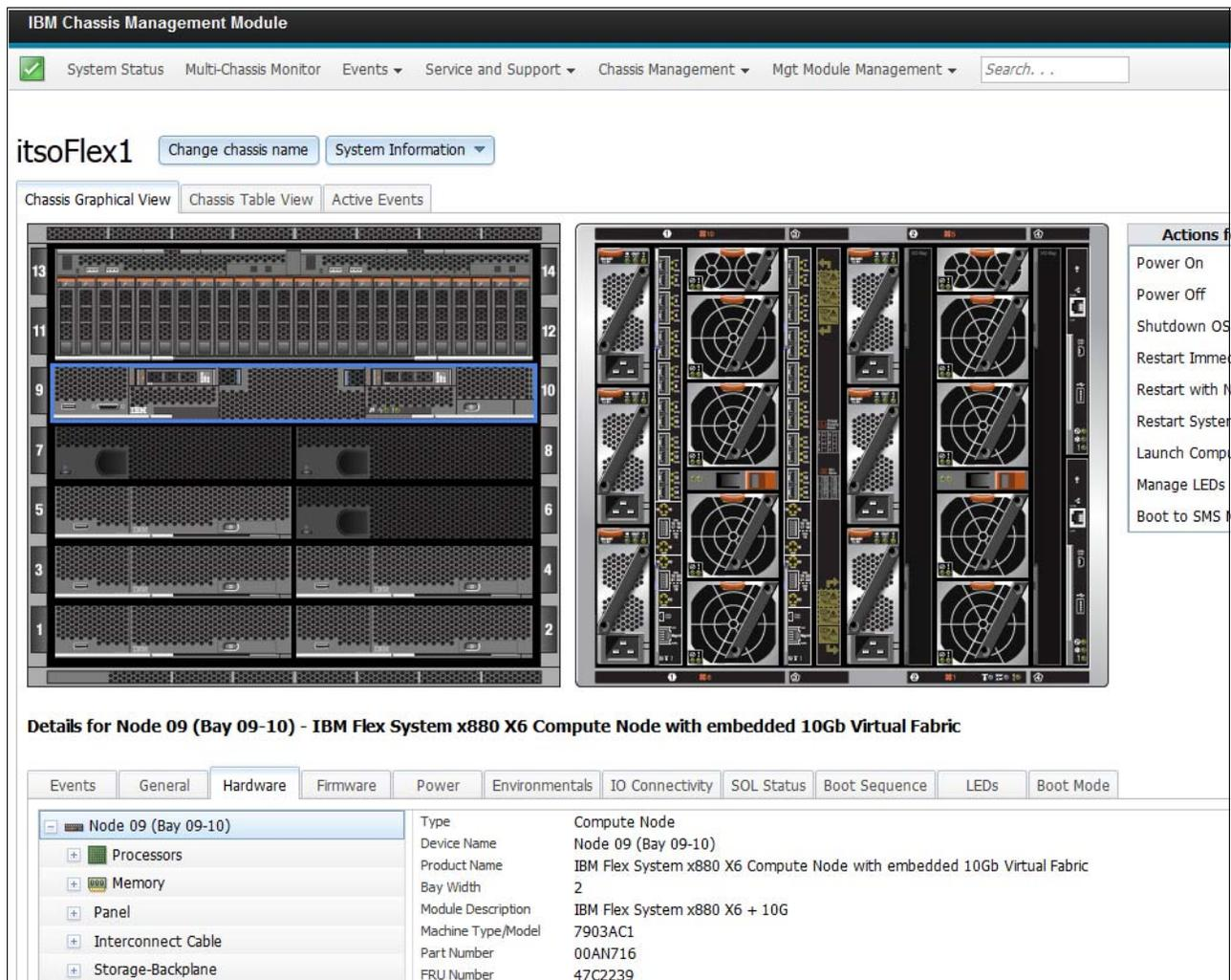
Figure 7-13 x880 compute node management options from System Status view
