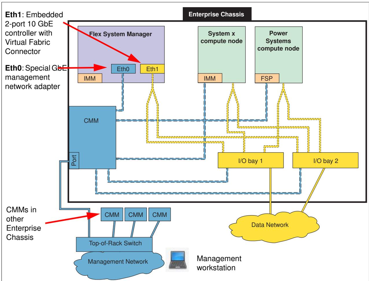
Figure 7-1 Separate management and production data networks
