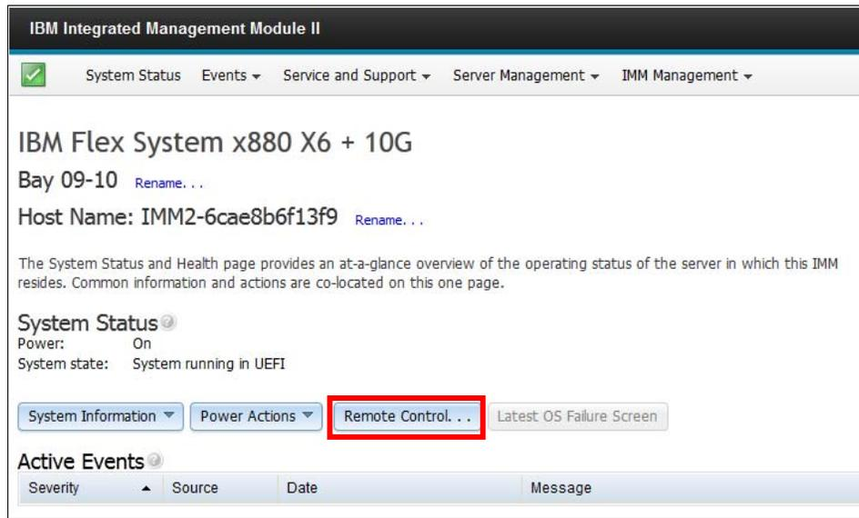
Figure 5-4 Remote Control button on the IMM2 main page
