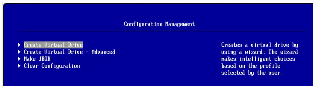
Figure 5-24 Configuration Management panel, Create Virtual Drive selected
