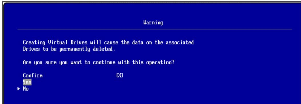
Figure 5-27 Warning and confirmation of RAID array creation
