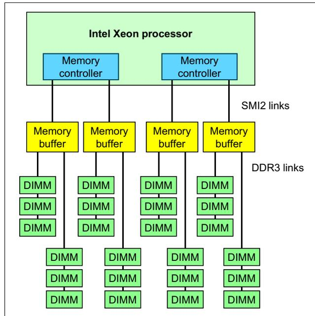
Figure 3-10 Intel Xeon processor E7 v2 memory architecture
