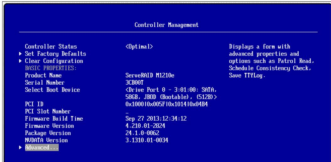
Figure 5-20 Controller Management panel, Advanced option selected
