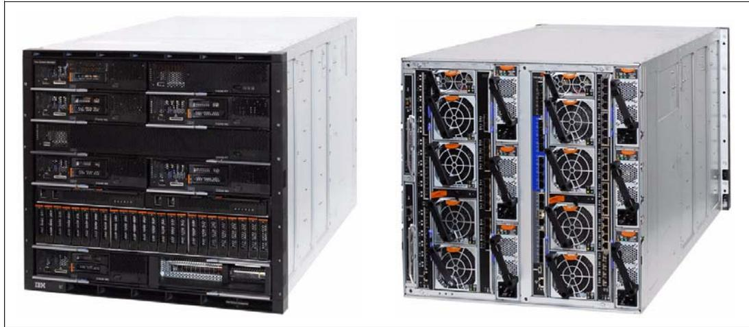
Figure 2-1 Lenovo Flex System Enterprise Chassis: Front and rear
