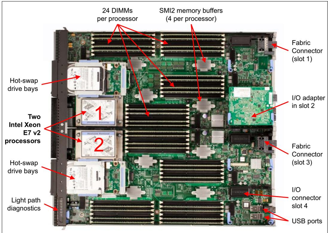
Figure 3-2 The Flex X6 Compute Node
