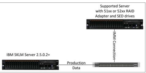
Figure 2-3 shows a minimum configuration that is required to test the basic functions.
