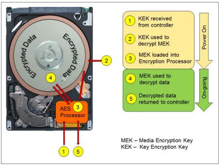
Figure 1-2 Secured SED drive boot process
