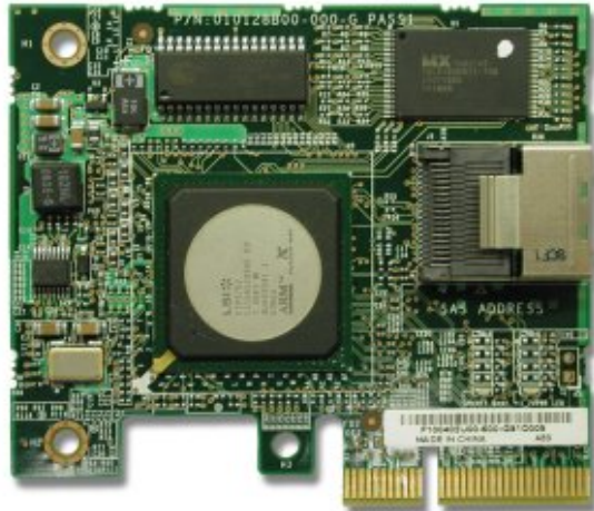
Figure 15. ServeRAID-BR10il SAS/SATA Controller v2 (BR10il v2)
