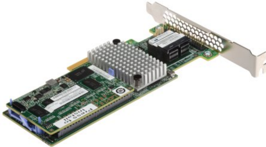
Figure 2. ServeRAID M5210 SAS/SATA Controller (with an optional cache installed)
