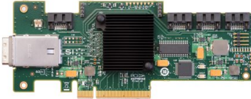
Figure 21. 6Gb SAS Host Bus Adapter with the PCIe slot bracket removed
