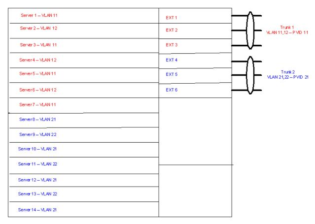
Example 3: Internal ports1.4 will be brought down when EXT1-3 are all down Internal ports 8-1.4 will be brought down when EXT4-6 are all down
