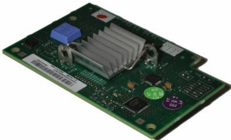
Figure 1. SAS Connectivity Card (CIOv) for BladeCenter
