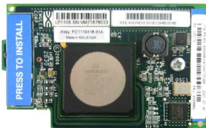
Figure 1. Emulex 4 Gb Fibre Channel Expansion Card (CFFv)
