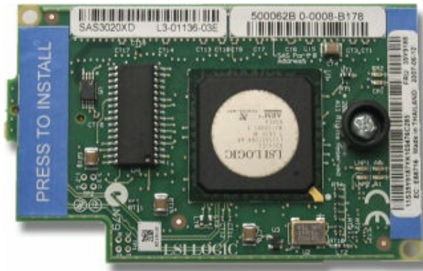
Figure 1. SAS Expansion Card (CFFv) for BladeCenter
