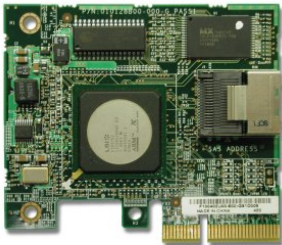
Figure 1. ServeRAID-BR10iL SAS/SATA Controller v2
