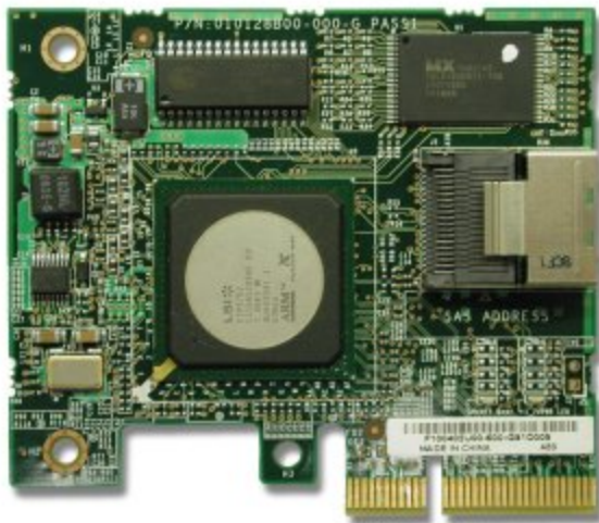
Figure 1. ServeRAID-BR10il SAS/SATA Controller v2
