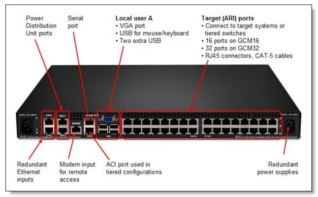
Figure 2. Connections on the GCM32 Global Console Manager
