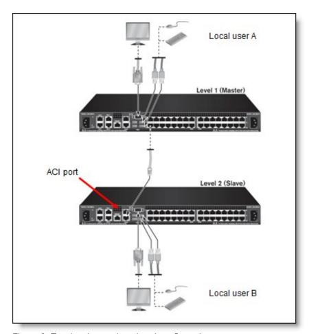
Figure 3. Two local users in a tiered configuration
