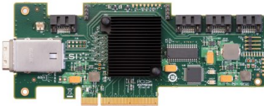
Figure 1. 6Gb SAS Host Bus Adapter
