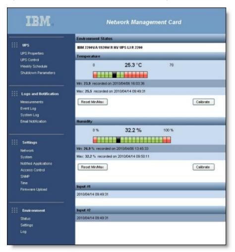
Figure 12. Environmental Monitoring Probe data as viewed from the Network Management Card web interface
