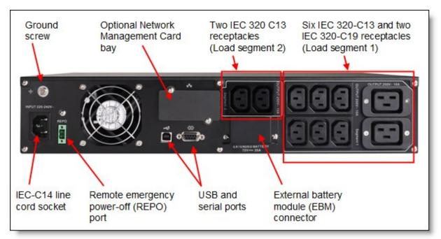
Figure 4. Rear panel of theIBM 2200VA LCD 2U Rack UPS (230V)
