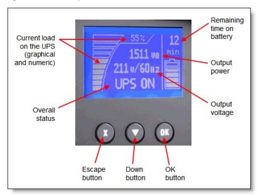
Figure 2. Front panel (showing System Status)
