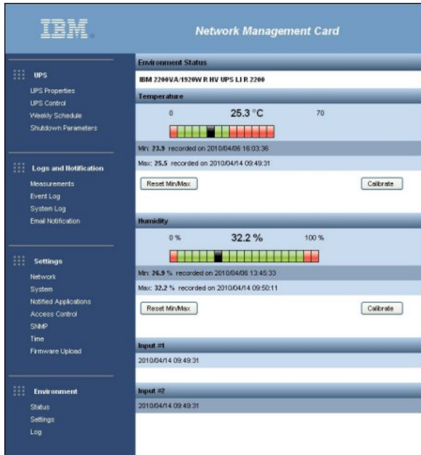
Figure 11. Environmental Monitoring Probe data as viewed from the Network Management Card web interface
