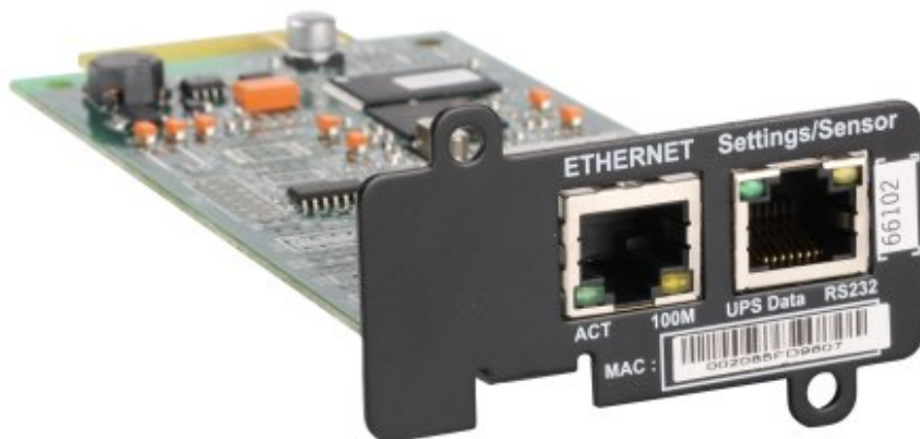
Figure 6. IBM LCD UPS Network Management Card (NMC)
