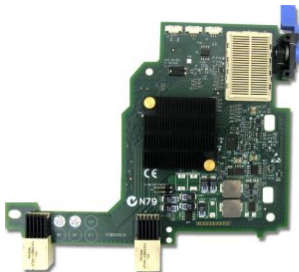
Figure 1. Mellanox 2-port 10Gb Ethernet Expansion Card (CFFh) for IBM BladeCenter
