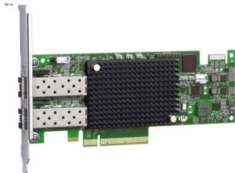
Figure 2. Emulex 16Gb FC Dual-port HBA (with 3U bracket attached; SFP+ are not present)
