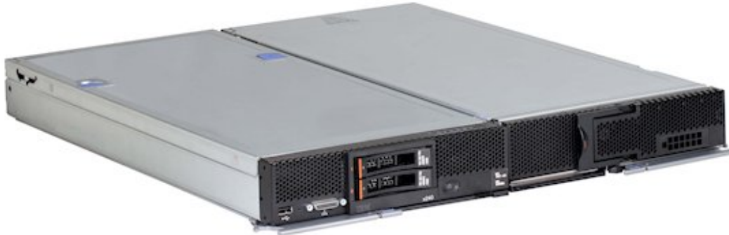
Figure 6. Flex System Storage Expansion Node (right) attached to a compute node (left)
