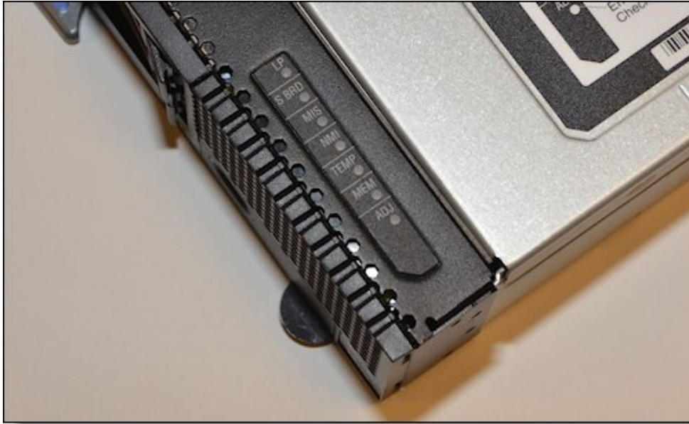
Figure 11. Location of x240 light path diagnostics panel
