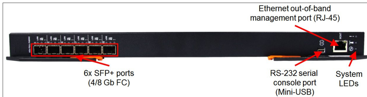
Figure 5. Front panel of the Flex System FC3171 8Gb SAN Switch and Pass-thru
