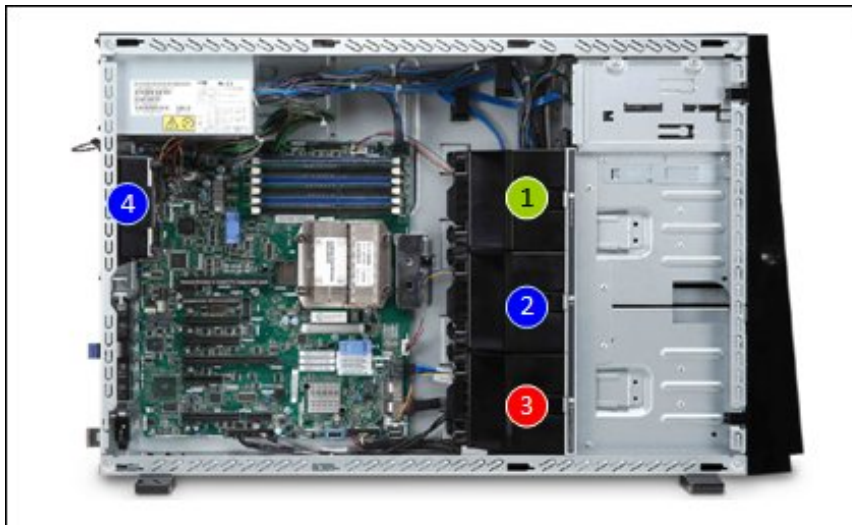
Figure 8. Location of the cooling fans
