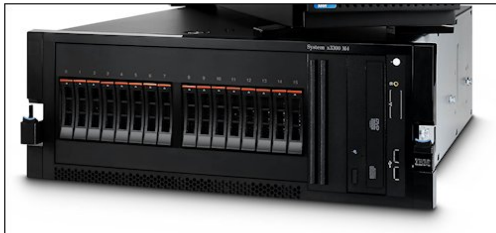
Figure 9. The System x3300 M4 server with the Tower to Rack Conversion Kit
