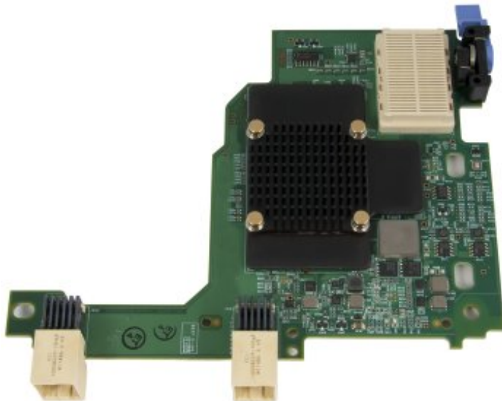
Figure 1. QLogic 10Gb Virtual Fabric Adapter for IBM BladeCenter
