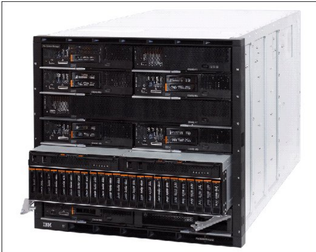
Figure 1. Front view of IBM Enterprise Flex System Chassis with IBM Flex System V7000 Storage Node
