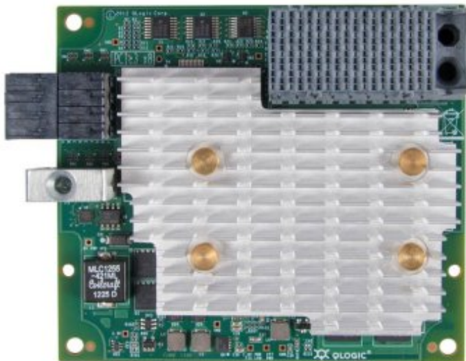
Figure 1. Flex System FC5172 2-port 16Gb FC Adapter
